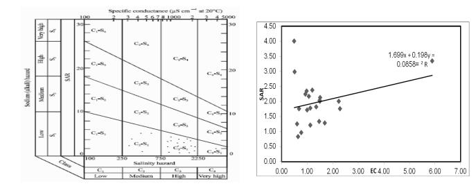
Fig.4. Wilcox diagram illustrating the suitability of groundwater in irrigation
