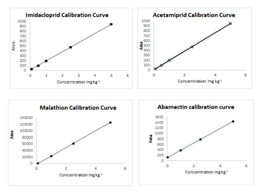
Fig (1) Calibration curves of imidacloprid, acetamiprid, malathion and abamectin
